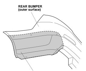
INSTALLATION POSITION Clean with isopropyl alcohol.
