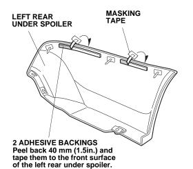
8. Using isopropyl alcohol on a shop towel, clean the surface where the left rear under spoiler will attach. Allow the surface to dry before going to the next step.
