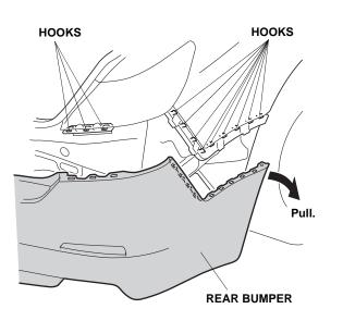
3. With the help of an assistant, remove the rear bumper (four hooks, and unplug the two vehicle connectors). Place the rear bumper on a blanket to prevent damage.
