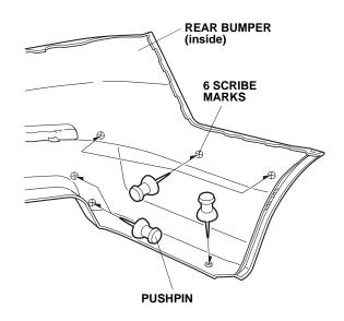
5. While wearing eye protection, drill the six pierced marks using a 3 mm drill bit, then finish with a 10 mm drill bit.
