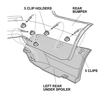
10. Secure the left rear under spoiler to the rear bumper with a bolt. Using a torque wrench, torque the bolt to 10 N·m (7.4 lbf·ft).
