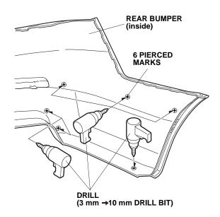
6. Using a deburring tool, remove any burrs from the holes.
